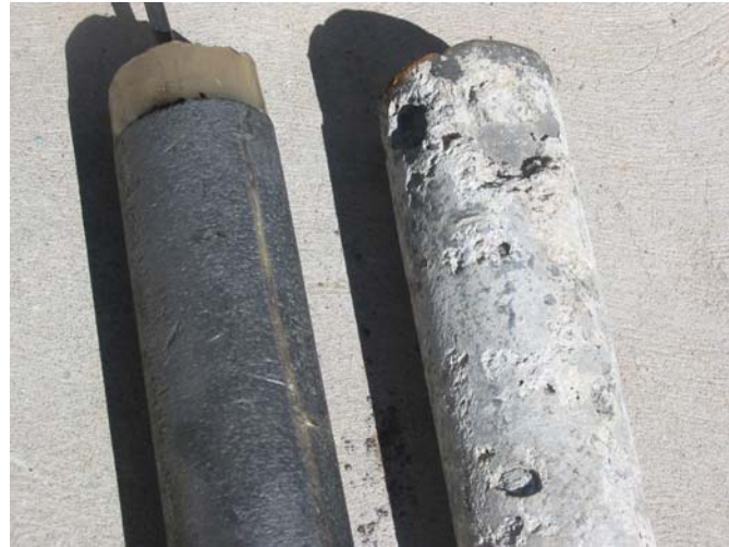
New Anode (left) Eroded Anode (right)
