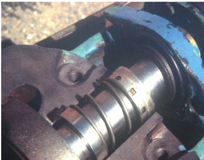
Mechanical Seal on a Horizontal Split Case Pump
